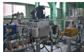
Hydrogen injection test bench
