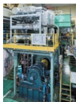
Ammonia fueled test engine
