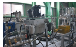
Hydrogen injection test bench
