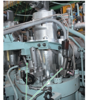
Fuel injection valves (Stratified injection)
