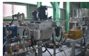
Hydrogen injection test bench
